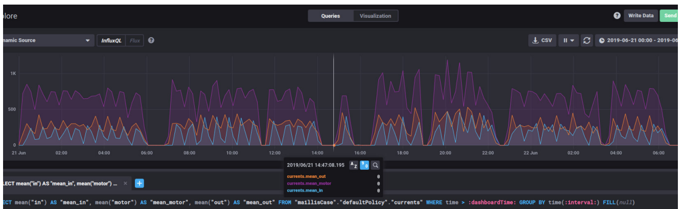
Figure 6: Retrieving Measurements of Current
