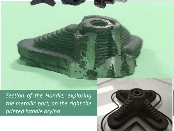
Section of the Handle, exposing the metallic part, on the right the printed handle drying
