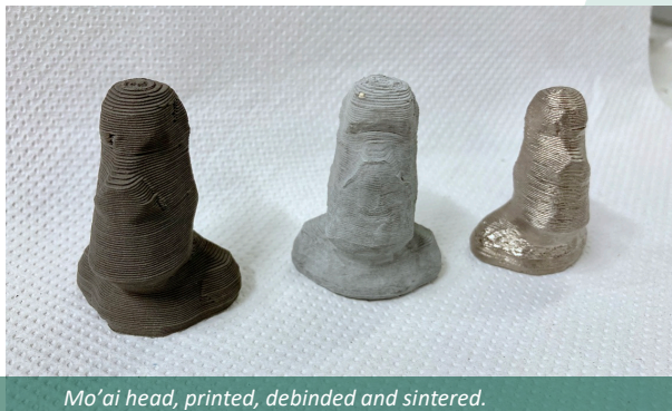
Mo'ai head, printed, debinded and sintered.
