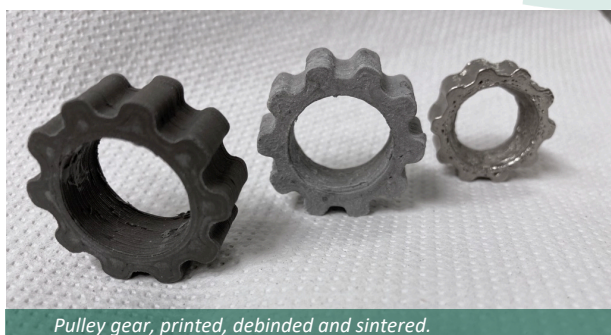
Pulley gear, printed, debinded and sintered.
