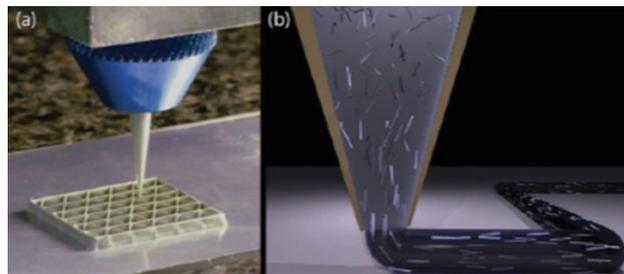
Figure 1. Principle of solid loaded DIW
