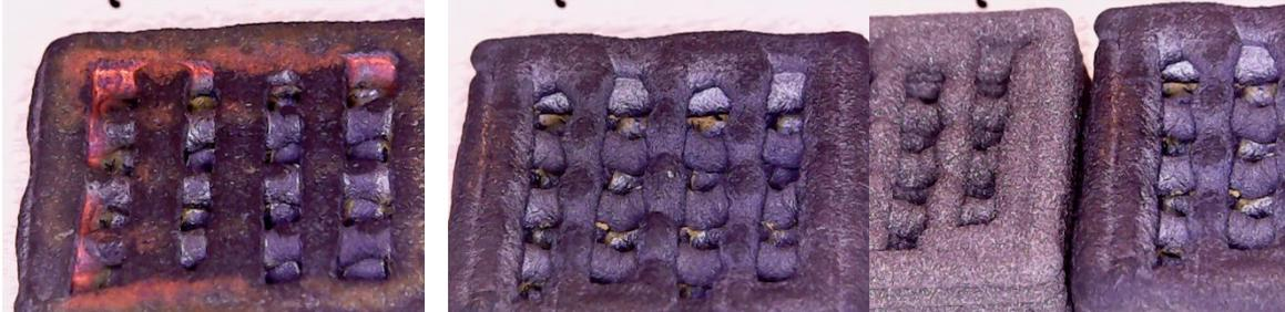
Figure 11. Result after the debinding and sintering process
