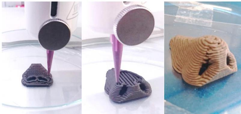
Figure 10. Nose structure printed using DIW technology with an iron based ink
