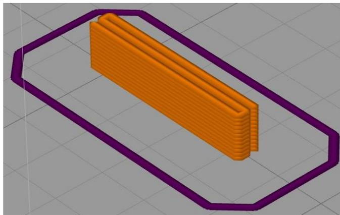
Figure 21. Path planning of the print of the sample with layers deposited in the long direction
