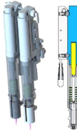
Figure 6. Concept design of the printer head
