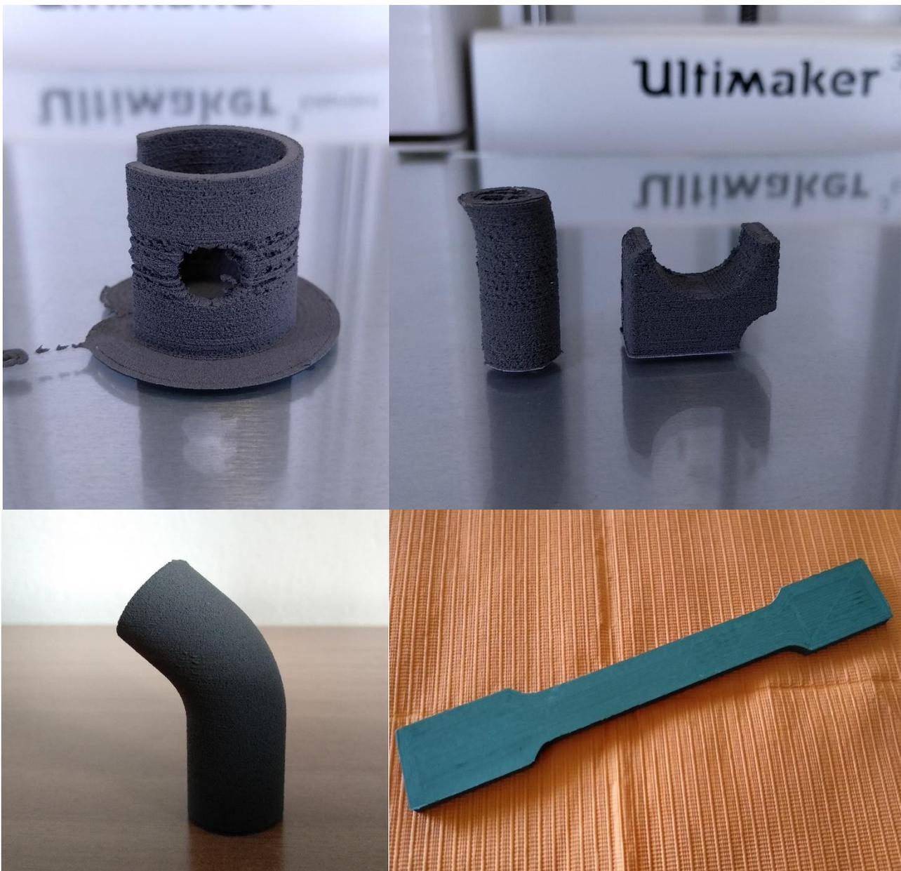
**Figure 26. Upper section: Unsuccessful 3D printing parts, Lower section: Successfully 3D printed parts using optimized parameters.**
