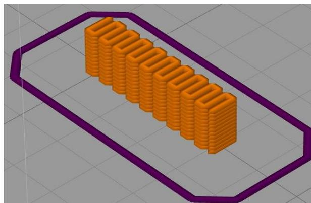
Figure 22. Path planning of the print of the sample with layers deposited in the short direction
