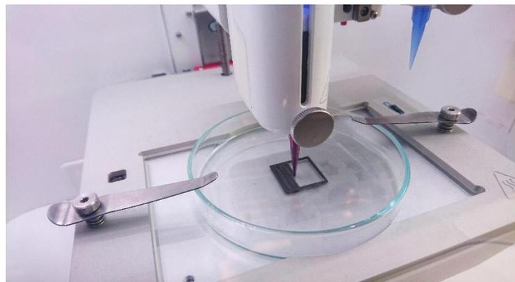
**Figure 3. BIO X 3D BIOPRINTER, printing low content solid loaded ink**
