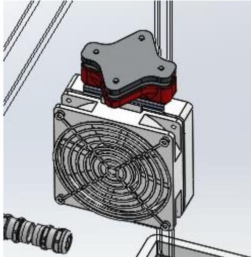
**Figure 19. Heater of the temperature control system**
