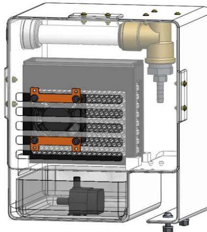
**Figure 20. Concept design of the humidity control system**
