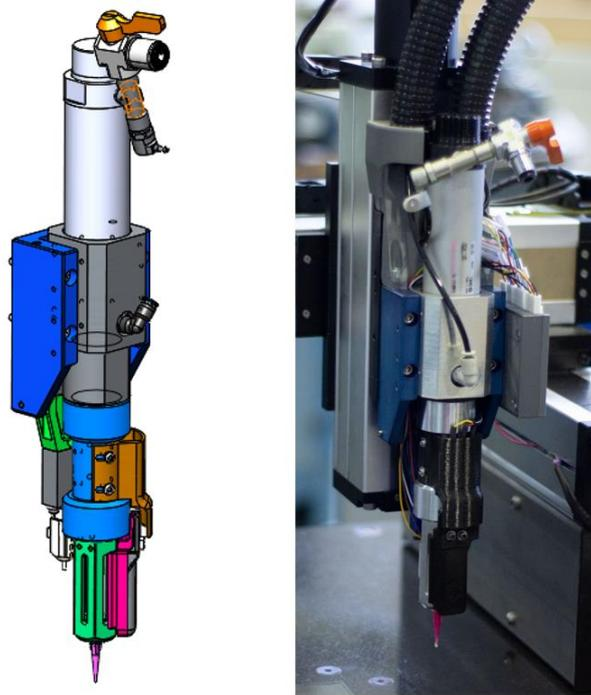
**Figure 16. Detail design and the result of the Printer Head**
