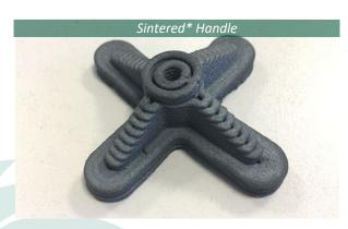
\*As sintered, without polishing or machining
