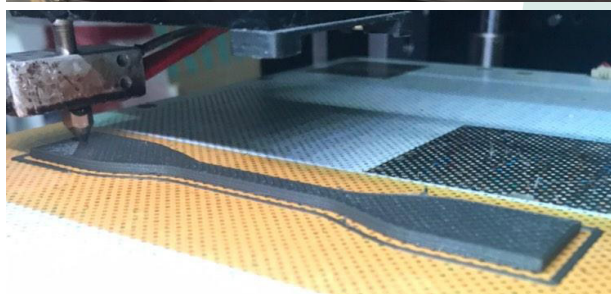
Dog-Bone specimen, being printed by 2 different printers
