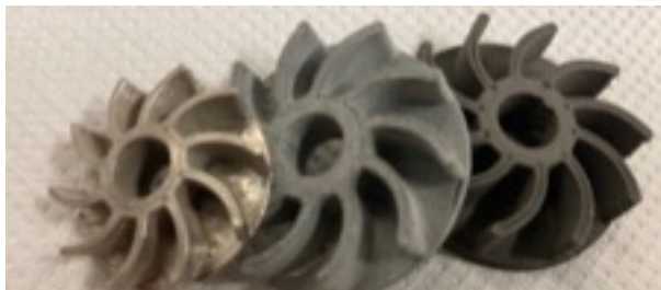
Impeller, printed debinded and sintered.
